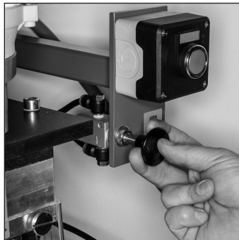
Clamp the hold-down devices.
