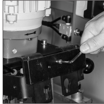
Side-to-side adjustment on ID arm plate.
