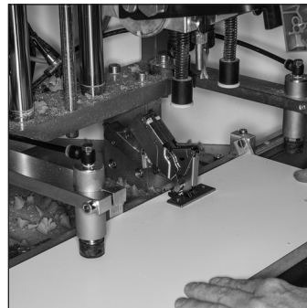
Pull hand lever up, remove workpiece.
