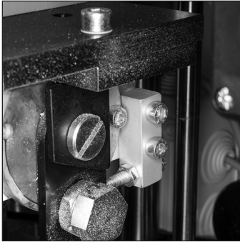
Hand lever adjusting screw. (front to back)
